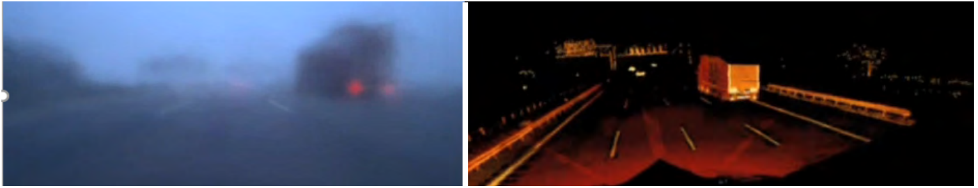
Figure 8: Camera vs. LiDAR in mist/rain
