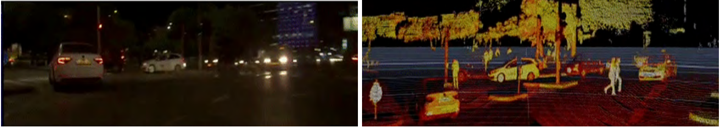
Figure 7: Camera vs. LiDAR in low-light conditions
