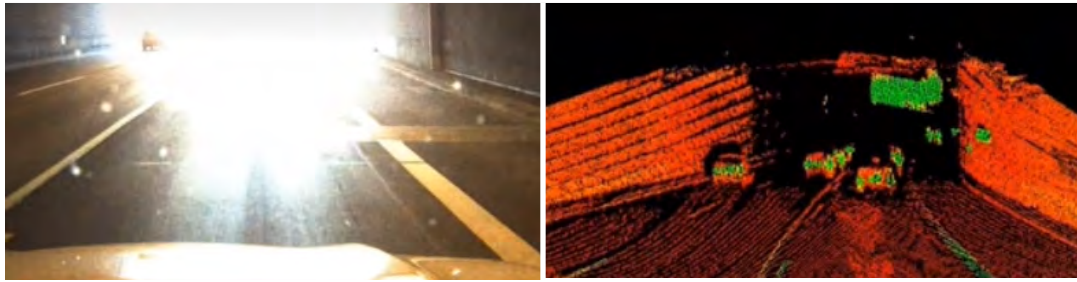
Figure 9: Camera vs. LiDAR in direct sunlight
